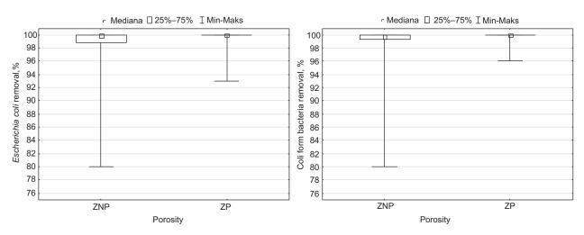
Fig. 3. Box-plot graphs of pathogenic bacteria removal on beds filled with porous (ZP) and non-porous material (ZNP)
