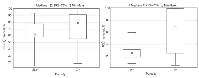
Fig. 2. Box-plot graphs of biogenic compounds removal on beds filled with porous (ZP) and non-porous material (ZNP)
