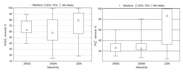
**Fig. 4.** Box-plot graphs of biogenic compounds removal on beds filled with non-selective plastic (ZNSS) and natural (ZNSN) material or selective natural material (ZSN)
