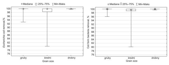
Fig. 7. Box-plot graphs of pathogenic bacteria removal on beds filled with coarse, medium and fine material
